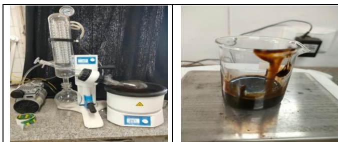
Figure 1. Extraction of laurel leaves by Soxhlet. Source: Own authorship.
